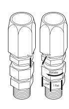
**Caution:** Do not introduce a twist to the hose when tightening the BP261 to the BP208 (or BP242).
