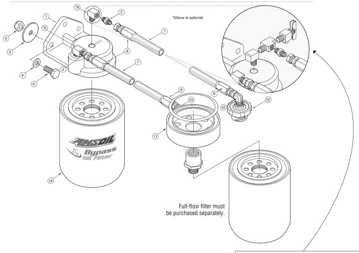
**Installing an oil sampling petcock:**Getting a clean and uncontaminated oil sample is easy and simple when an oil sampling petcock is installed into a Bypass Oil Filter system. This can be easily done by ordering a BP67 Kit and installing it into the bypass system as shown here.
